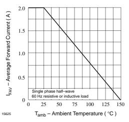
Figure 1. Max. Average Forward Current vs.
