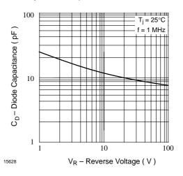
Figure 4. Typ. Diode Capacitance vs. Reverse Voltage
